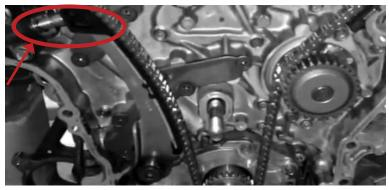
Correct alignment of tensioner and chain guide.
