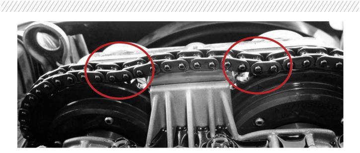
If the chain looks like the above circled areas, it is time to replace the timing components. Notice how the chain sags. This should not occur in any location of the chain drive. If slack is present replace the chain, chain tensioner, and chain guides.
